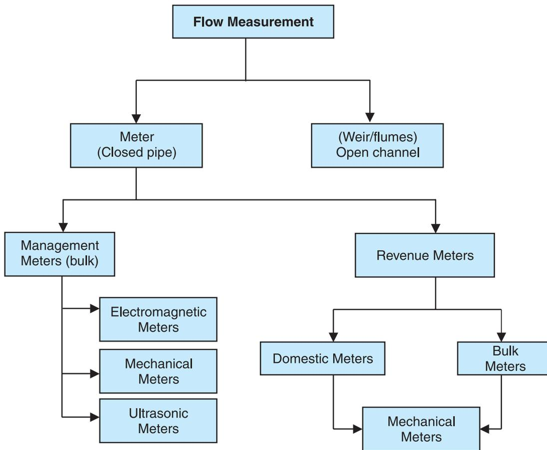
**Figure 1** Types of flow meters
