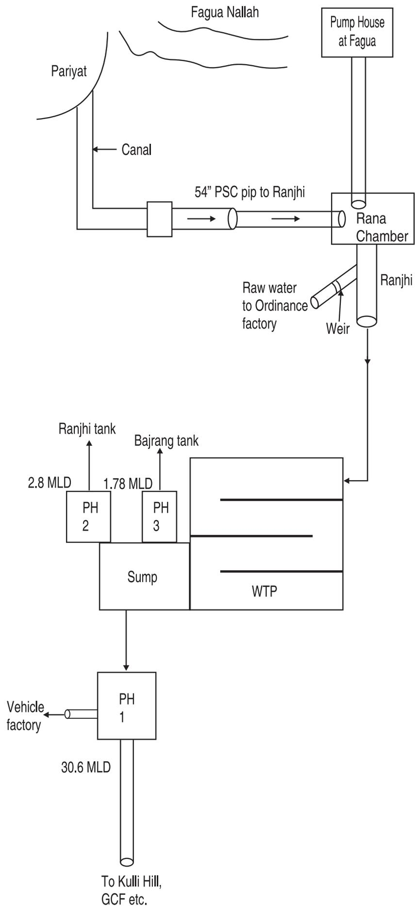
**Figure 2.3** Pariyat-Fagua system (Ranjhi treatment plant)
