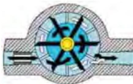
**Figure 4** Rotary vane flow meter
