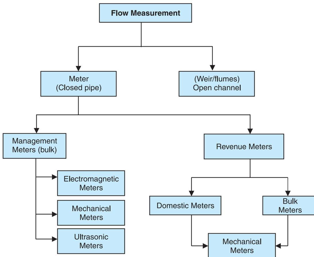
**Figure 1** Types of flow meters
