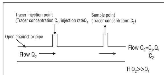
**Figure 1** Dilution gauging by tracer injection
