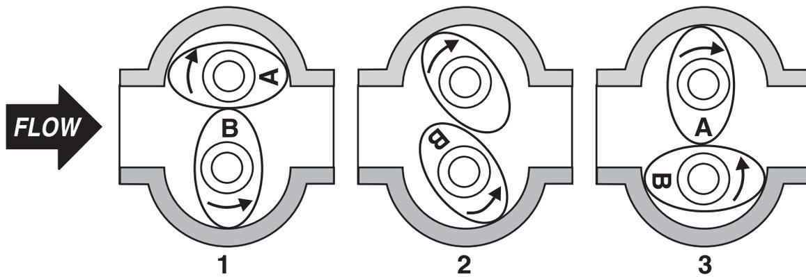
**Figure 3** Oval gear flow meter
