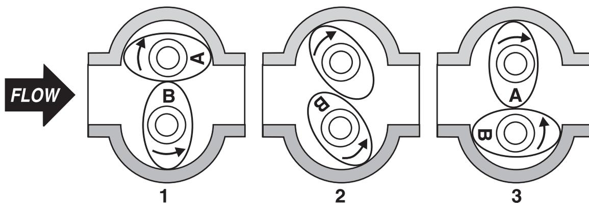
**Figure 3** Oval gear flow meter
