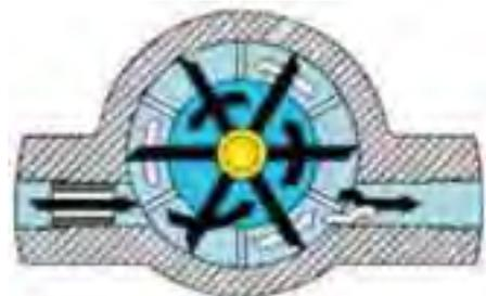
**Figure 4** Rotary vane flow meter
