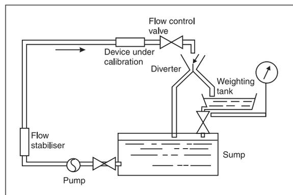
**Figure 2** Flow calibration by weighing
