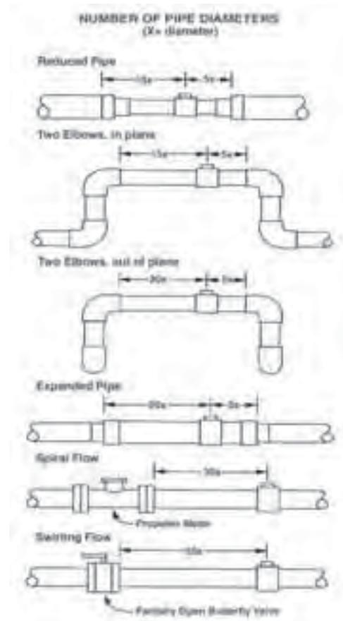
Figure 3 Different alignments for positioning of flow meter
