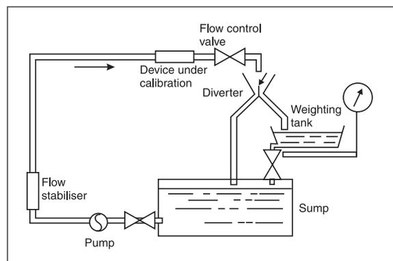
**Figure 2** Flow calibration by weighing
