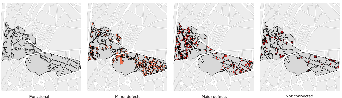
Figure 46 Condition of buildings' connection to stormwater network
