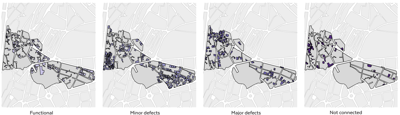
Figure 44 Condition of buildings' connection to wastewater network
