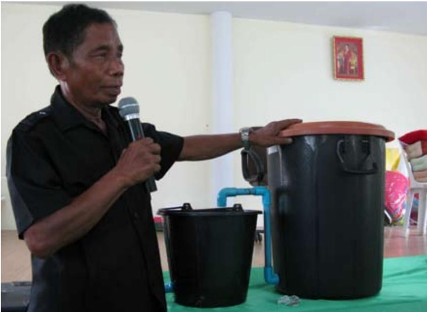
The kitchen grease filtration system being demonstrated.
