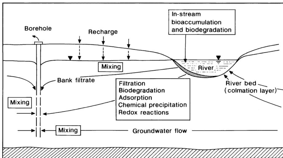
Figure 1: Basic scheme of riverbank filtration and main attenuation processes [1]
