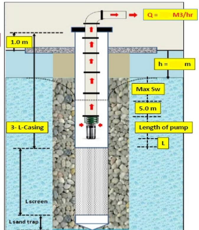
Figure 56: Typical RBF well components
