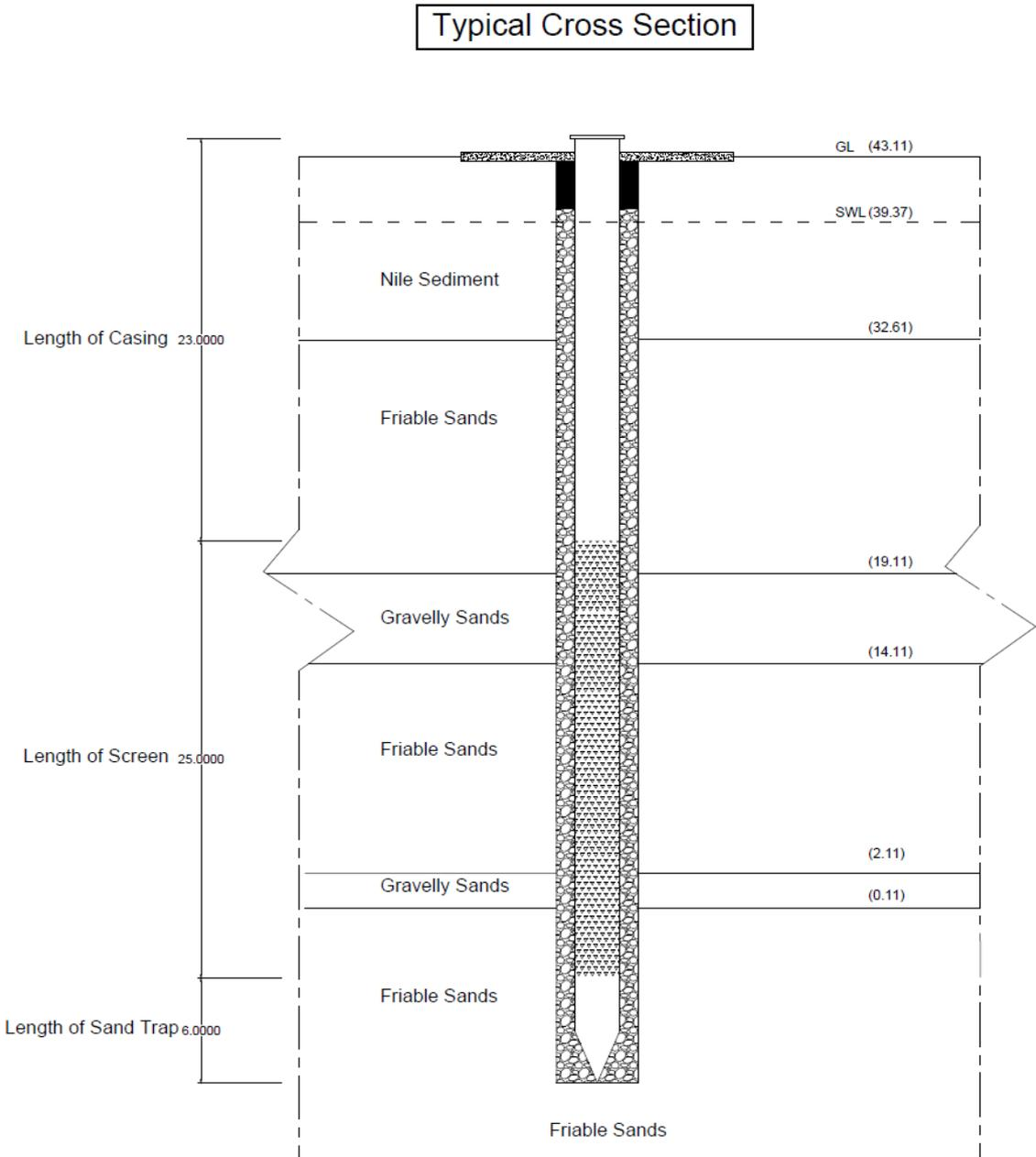
Figure 58: Typical well profile – Cross section, Levels provided as a rough guide
