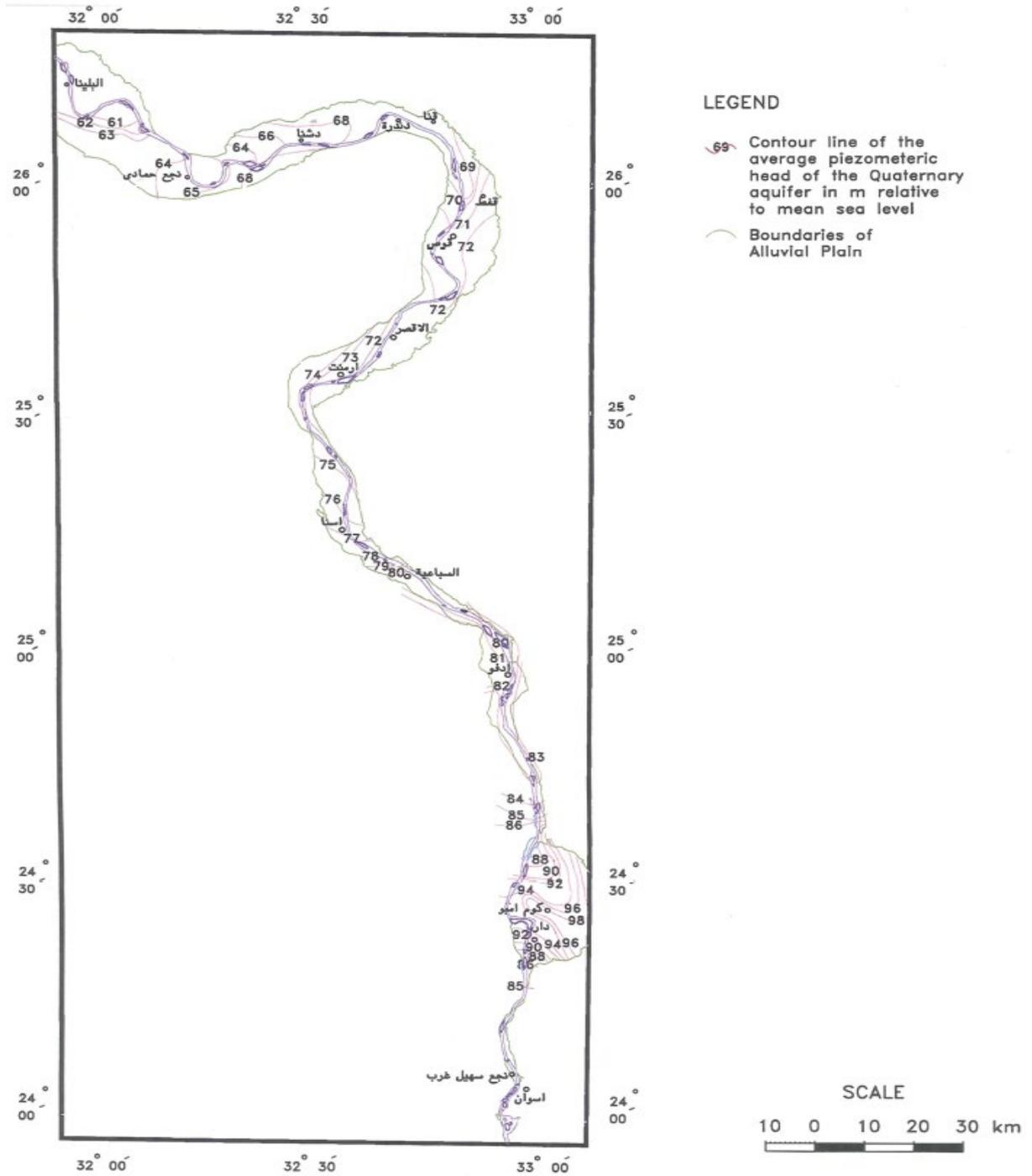
Figure 11: Aquifer piezometric contour lines - Upper Egypt [11]
