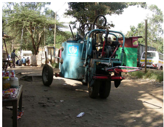
Photo 3: The UN-Habitat suction device is used for evacuating pit latrines but it cannot work where access is limited.
