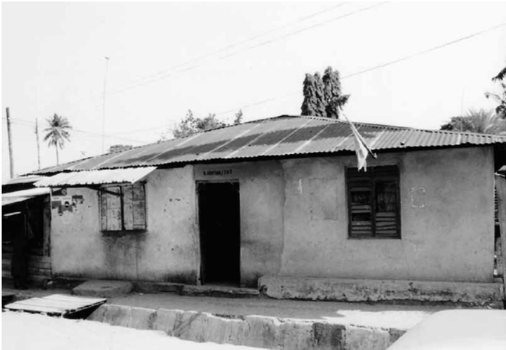
The modern Swahili type in Dar es Salaam is usually built with a proper foundation made of concrete or other durable material such as stone, its walls are made of sand cement blocks
