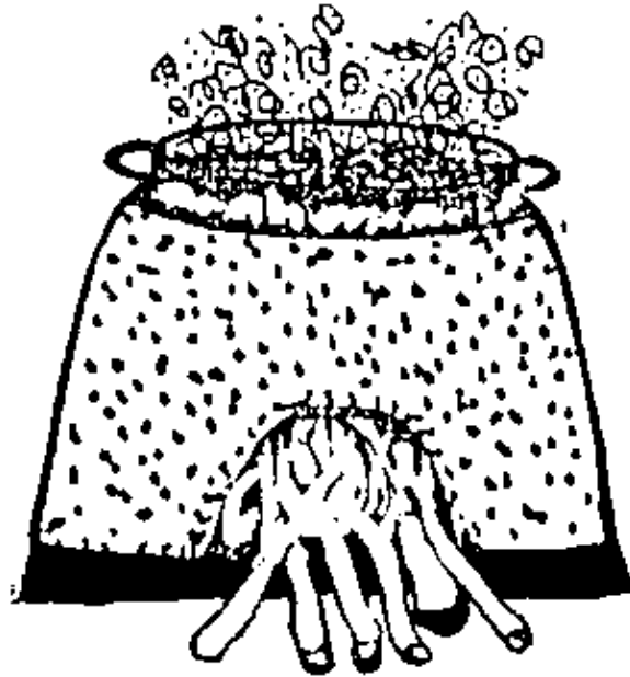
Figure 10. The improved three–stone stove ( trois pierres améliorées ) (3PA)
