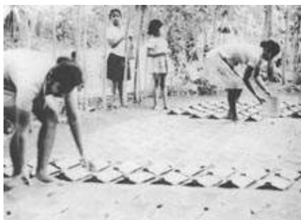
Figure 2.8. Energy consumption in brick and tile manufacture can be reduced by making use of solar energy for drying the units before they are loaded into the kiln (Yogyakarta Province, Indonesia).
