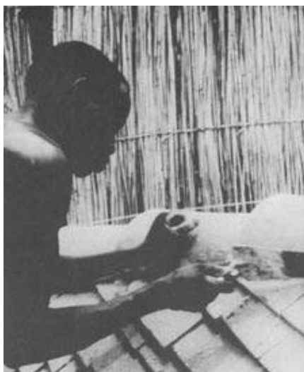
Figure 3.8. Clay tiles are simple to manufacture, but the energy required for firing them makes them more energy-intensive, per area of roof, than concrete or fibre-concrete tiles.
