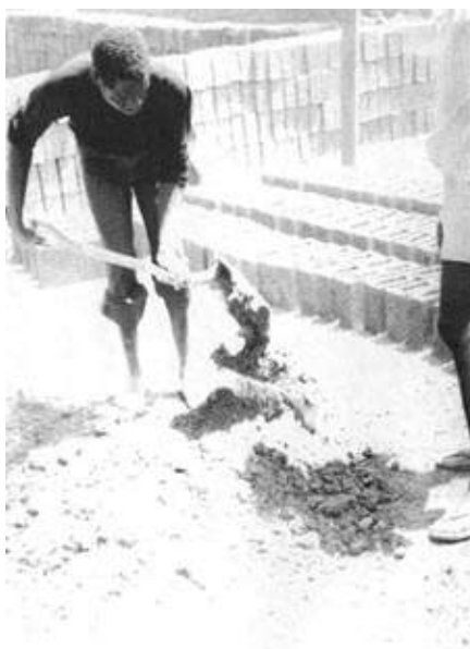
Figure 2.12. Stabilized soil blocks can also be made using manual compaction. The energy requirement is lower, because less equipment is needed (Lusaka, Zambia).
