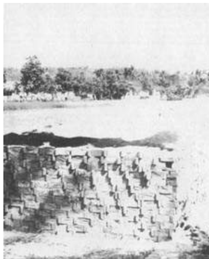
Figure 2.7. Rice husk is frequently available as a waste material in rice-growing areas, but can be used as a fuel for firing bricks, as shown here in Indonesia.
