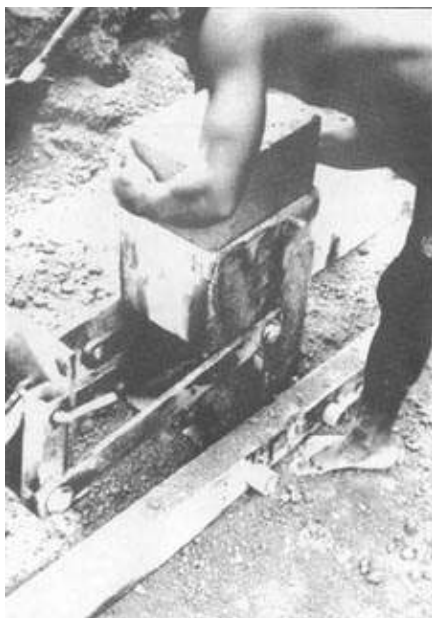
Figure 2.11. Stabilized-soil blocks can be made in a manually-operated press. Stabilized with 5 per cent cement they have an energy requirement for lower than burnt clay bricks or concrete blocks (Kumasi, Ghana).
