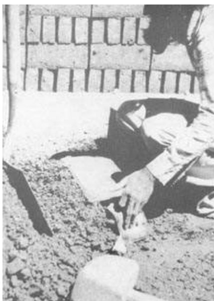
Figure 2.14. In volcanic areas, lime-trass blocks can be made with properties similar to concrete blocks, but eliminating the need for cement altogether. These blocks are made from a mix of 1 part lime to 5 trass, and they use less energy than concrete blocks (Bandung, Indonesia).
