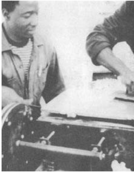
Figure 3.6. Fibre-concrete tiles are one of the most energy-efficient of the permanent roofing materials. They can be made on a small scale with little equipment and no purchased power.
