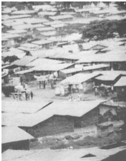
Figure 3.7. Steel sheets, even though thin and light in weight, embody a considerable amount of energy. They have an energy content per unit area of roof over 15 times that of fibre-concrete tiles.
