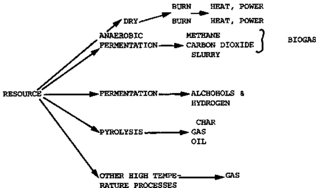
Figure 4. Technological options for converting organic matter into energy.
