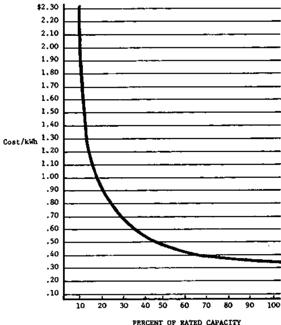
Fig. 3. Variation of cost per kilowatt with power factor for a 8 kWh diesel generator (cost of fuel, \$ 1.50 per gallon).
