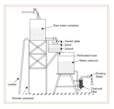
and the water in the tank is stirred and the flow is drained through the cock which is at the bottom. Then the tap is opened and water flows onto the swash plate in the second container until the tank is full. The outlet tap allows water to flow through a charcoal filter contained in a cylindrical vessel about 75 cm in length and 25 cm
