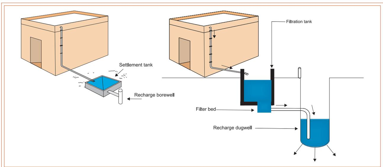
The above figures show typical systems of recharging wells directly with rooftop runoff. Rainwater that is collected on the rooftop of the building is diverted by drainpipes to a settlement or filtration tank, from which it flows into the recharge well (bore well or dug well).
