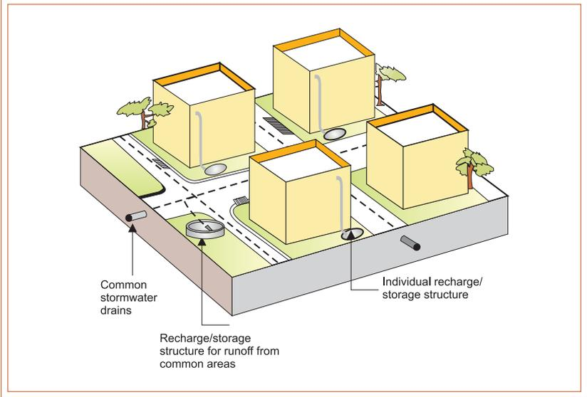
Trapping storm water drains in a community-level system
