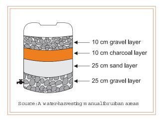
Sand filters are commonly available and are easy and inexpensive to construct. These filters can be employed for treatment of water to effectively remove turbidity (suspended particles like silt and clay), colour and microorganisms.
