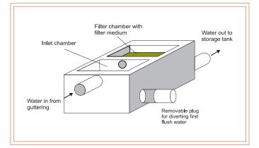
rainwater tank. This is sealed at the bottom with a plug. When rain begins to fall, this length of pipe must fill before any water can enter the tank. It will, thus, retain any sediment carried by the first flush water. After each storm, the plug is removed and the pipe is drained. Also consider trimming any tree branches that overhang the roof. These branches are perches for birds and produce leaves and other debris.
