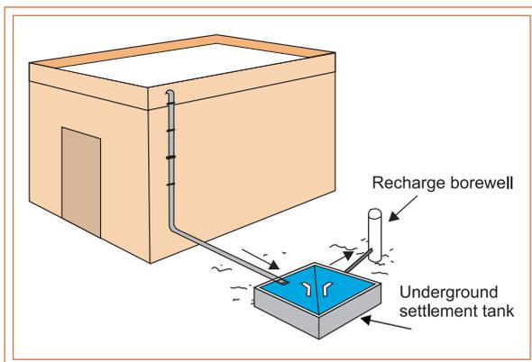
Recharge pits are constructed for recharging the shallow aquifers. These are constructed generally 1 to 2 m. wide and 2 to 3 m. deep. After excavation, the pits are refilled with pebbles and boulders as well as coarse sand. The construction details are given in the drawing below.
