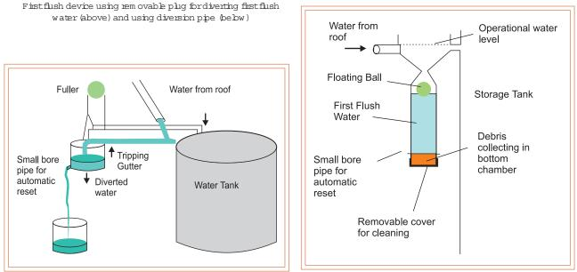
The Tripping Gutter first-flush system
