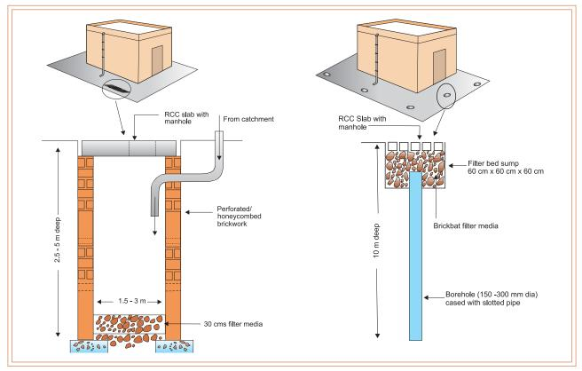
Location of mechange pit in a building area and detailed section of pit
