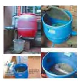
Drum s - Filters and interm ediate storage segregator
