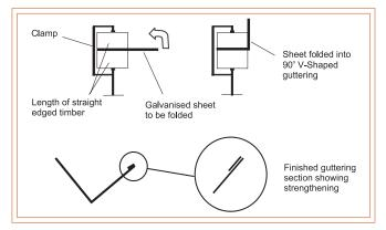
Folding galvanised steelsheet to make V-shaped guttering
