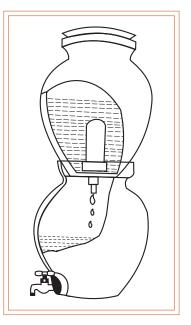
electrolytes. Candles are made by the usual casting process with plaster of paris moulds. These are finished and baked at a suitable temperature. Candles are then given a special chemical treatment so that they can give bacteria free water. The life of a candle is generally 2 - 3 years and can be installed in any domestic container.
