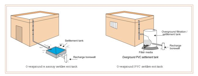
Apart from removing silt from the water, the desilting chamber acts like a buffer in the system. In case of excess rainfall, the rate of recharge, especially of bore wells, may not match the rate of rainfall. In such situations, the desilting chamber holds the excess amount of water till it is soaked up by the recharge structure.
