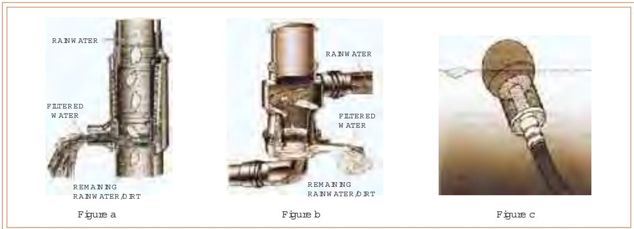
Figure a: A filter collector diverts 90 per cent of rainwater to a storage tank through a 0.17 mm stainless steel mesh filter.
