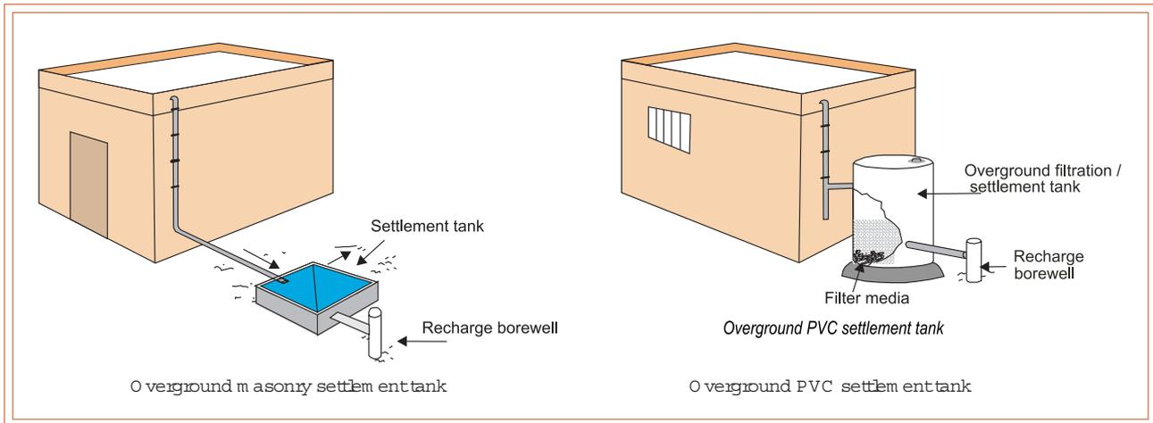
Apart from removing silt from the water, the desilting chamber acts like a buffer in the system. In case of excess rainfall, the rate of recharge, especially of bore wells, may not match the rate of rainfall. In such situations, the desilting chamber holds the excess amount of water till it is soaked up by the recharge structure.
