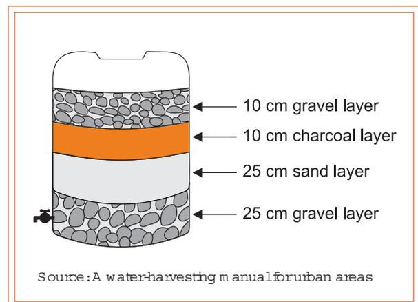
Sand filters are commonly available and are easy and inexpensive to construct. These filters can be employed for treatment of water to effectively remove turbidity (suspended particles like silt and clay), colour and microorganisms.
