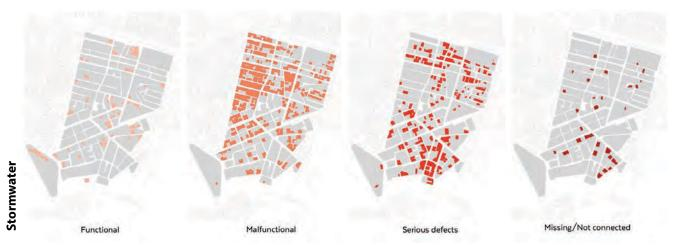
Figure 19 Building connection to stormwater network
