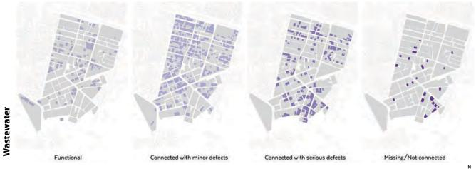
Figure 16 Building connection to wastewater network
