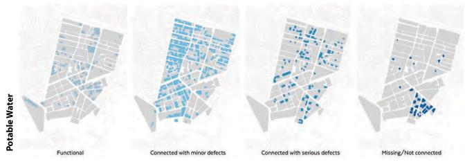
Figure 15 Building connection to potable water network
