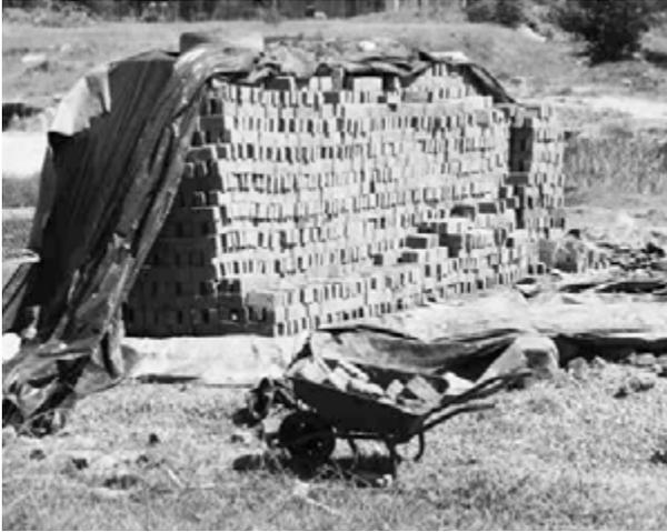
FIGURE 79 A clamp of about 12,000 bricks during their burning, Maseru East
