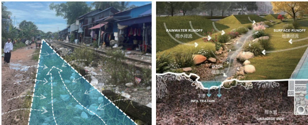
Figure 3.9 Schematic Diagram of Ecological Ditch Renovation
