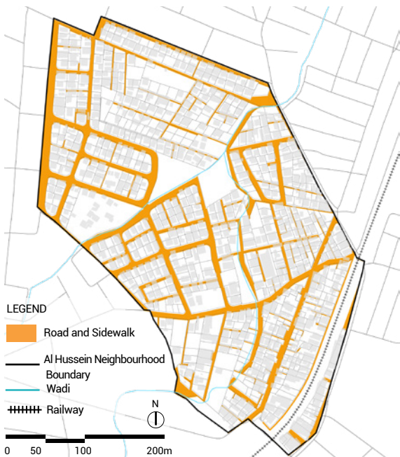
Fig. 33: Road & Sidewalk Networks' Upgrading Project
