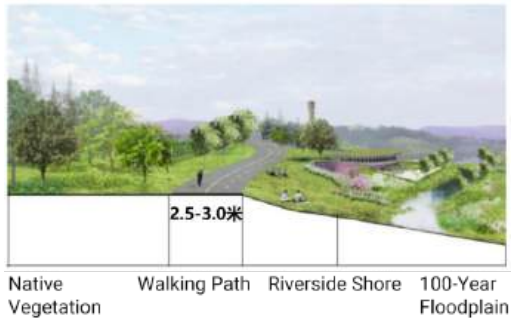
Figure 71: Cross Section of the Pedestrian Pathway with Recreational Elements
