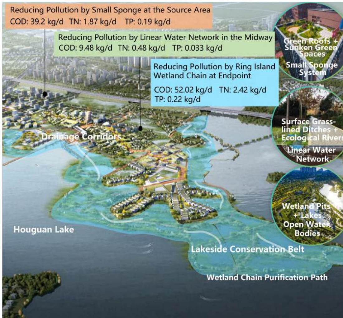
Figure 67: Schematic Diagram of the Multi-stage Ecological Pollution Interception and Purification System
