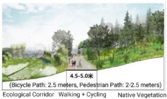
Figure 69: Cross Section of the Main Commuting Greenway
