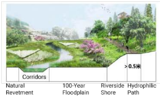
Figure 73: Cross Section of the Main Recreational Pathway
