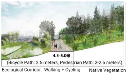
Figure 59: Cross Section of Main Greenway
