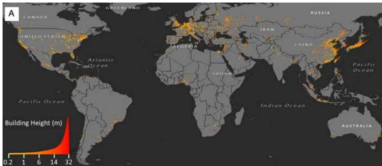
Figure 6.4: Global urban built-up heights derived from satellite observations [the colour and height of the bar represent built-up heights in each 500m grid]
