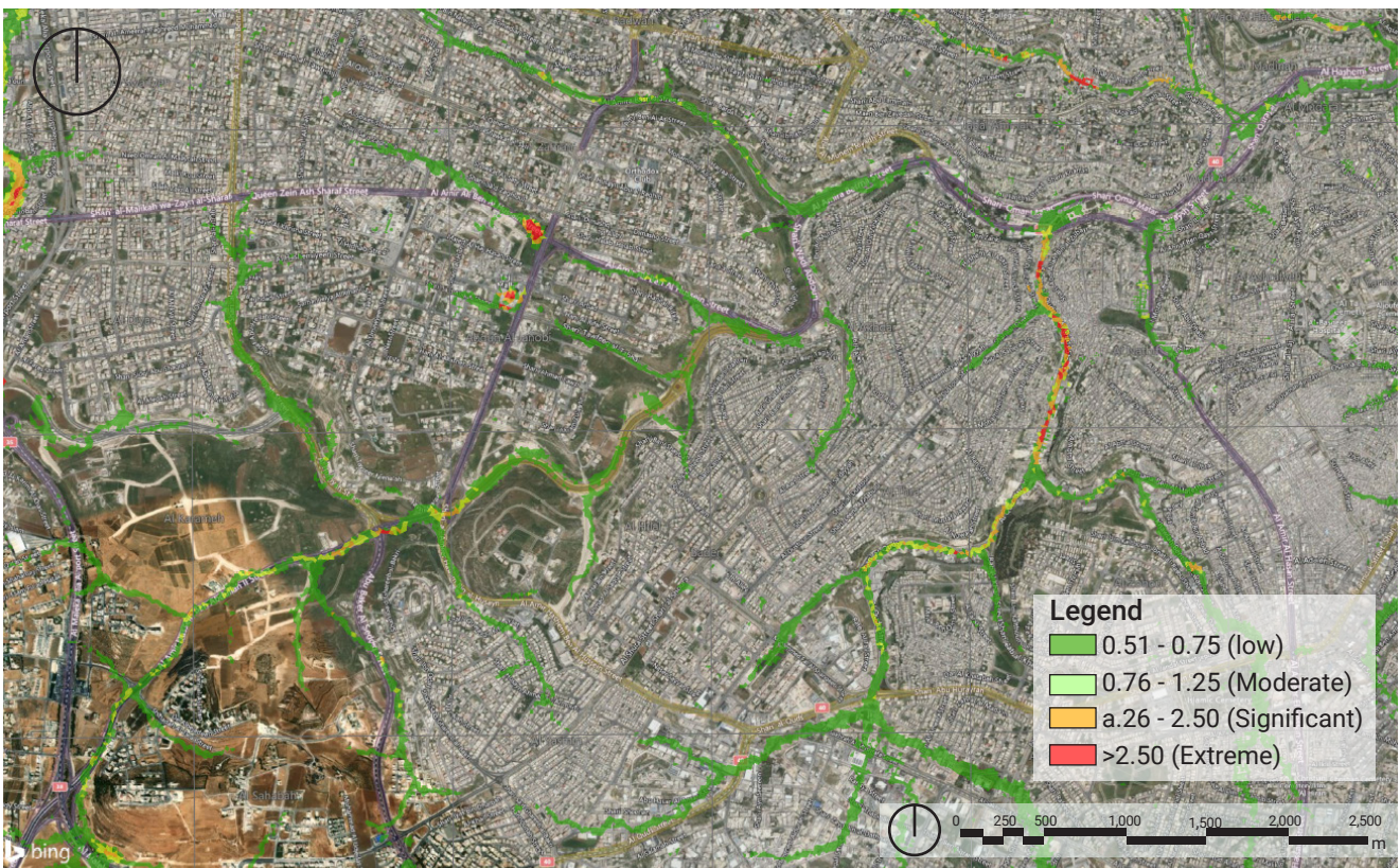
Fig. 10: Hazard map for the 2 year flooding event.
