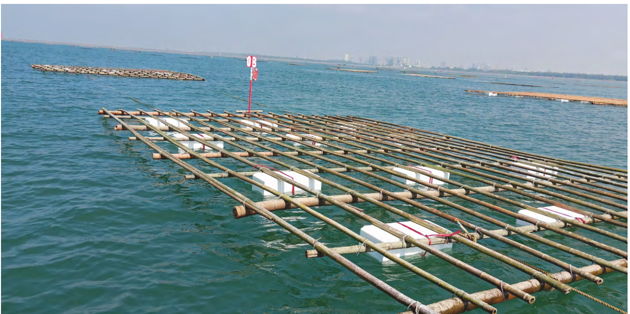
△ EPP Foamable Polypropylene Floating Gear Sea Trial Experiment
