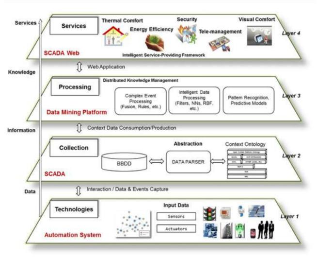
Figure 2-1 common architecture of smart building management system (Moreno et al. 2014) Source: Sensors,2014,14(6).
