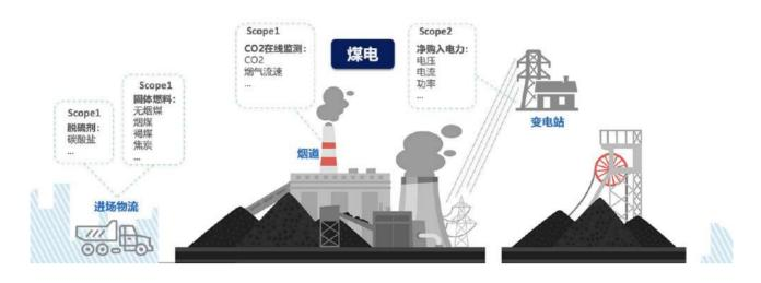
Figure 3-3: diagram of carbon emission monitoring in the coal power (energy) sector Source: draw by author
