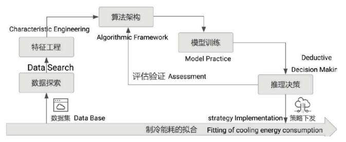
Figure 3-9: High efficiency refrigeration control strategy Source: Next Generation Data Center White Paper, Huawei
