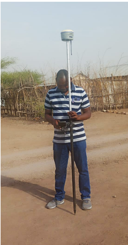
The technical team collecting spot heights during the site visit. © UN-Habitat
