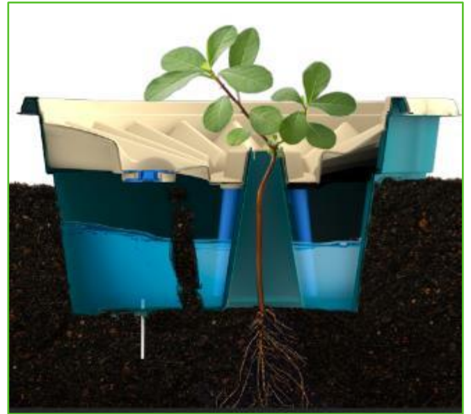
Image 95: Installation of Ekobox ® in areas with irrigation challenges
