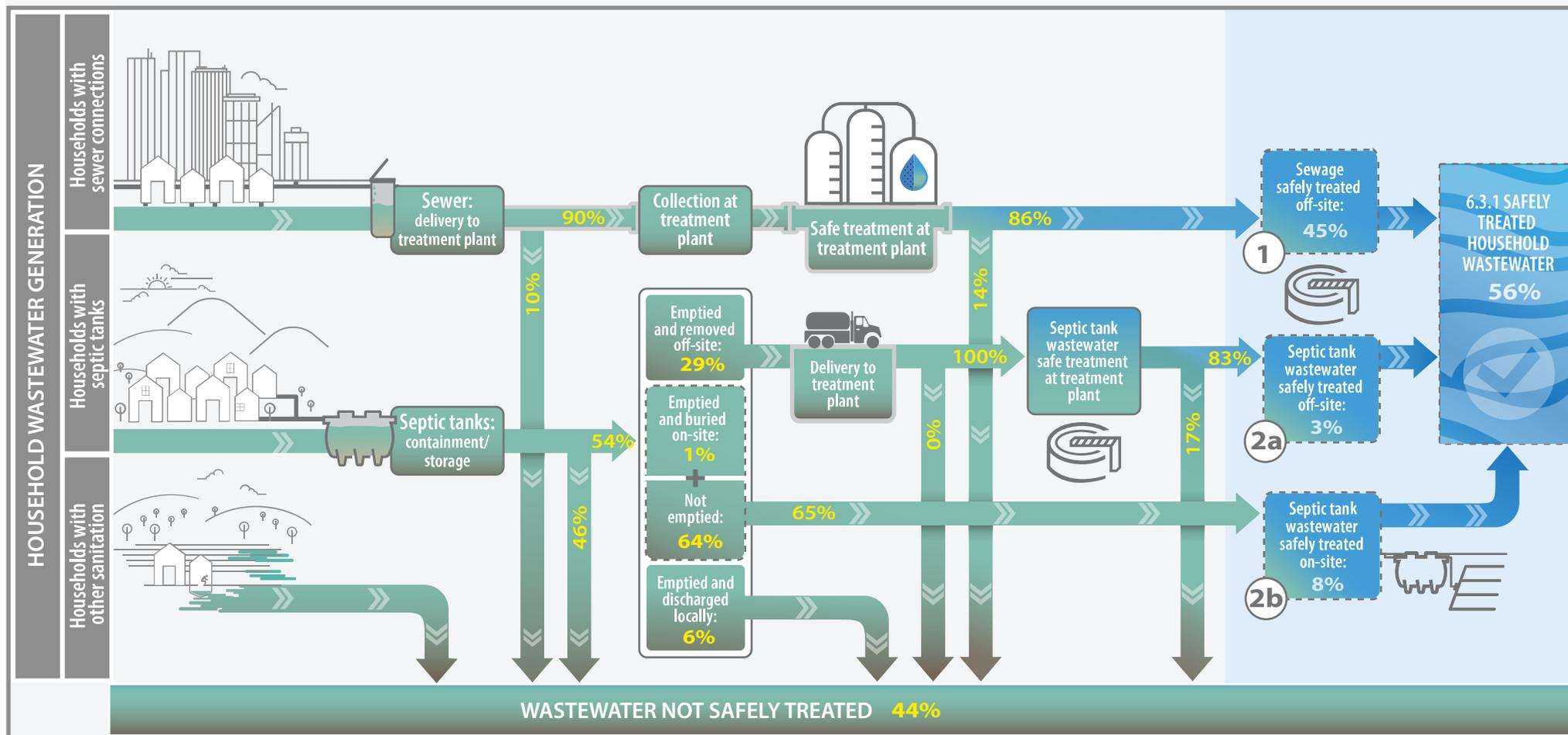
**Figure 22. Safely treated sewer wastewater flows determined based on compliance or technology (2020)**
