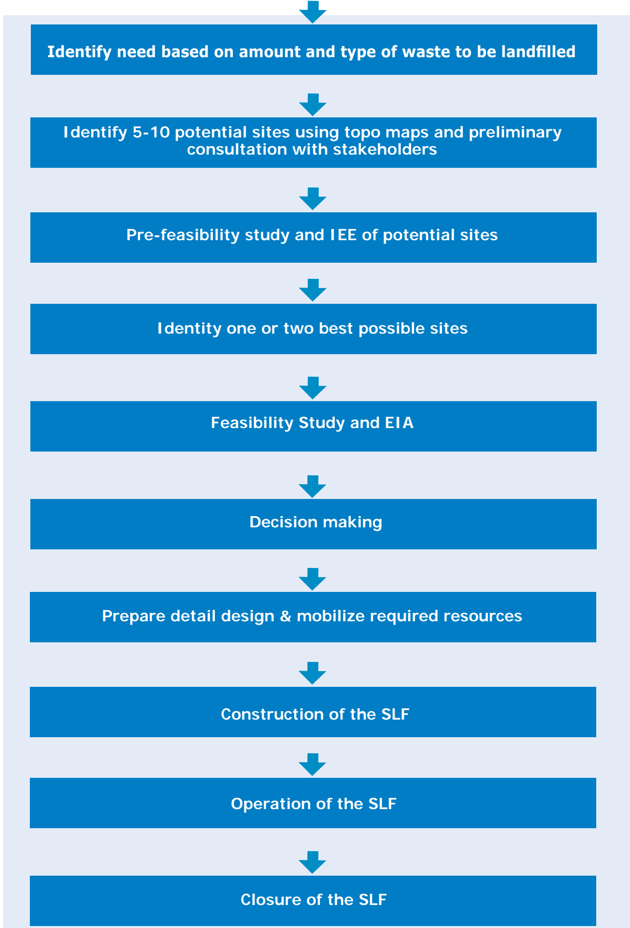
Figure 6.9: Process of Landfill Development and Operation
