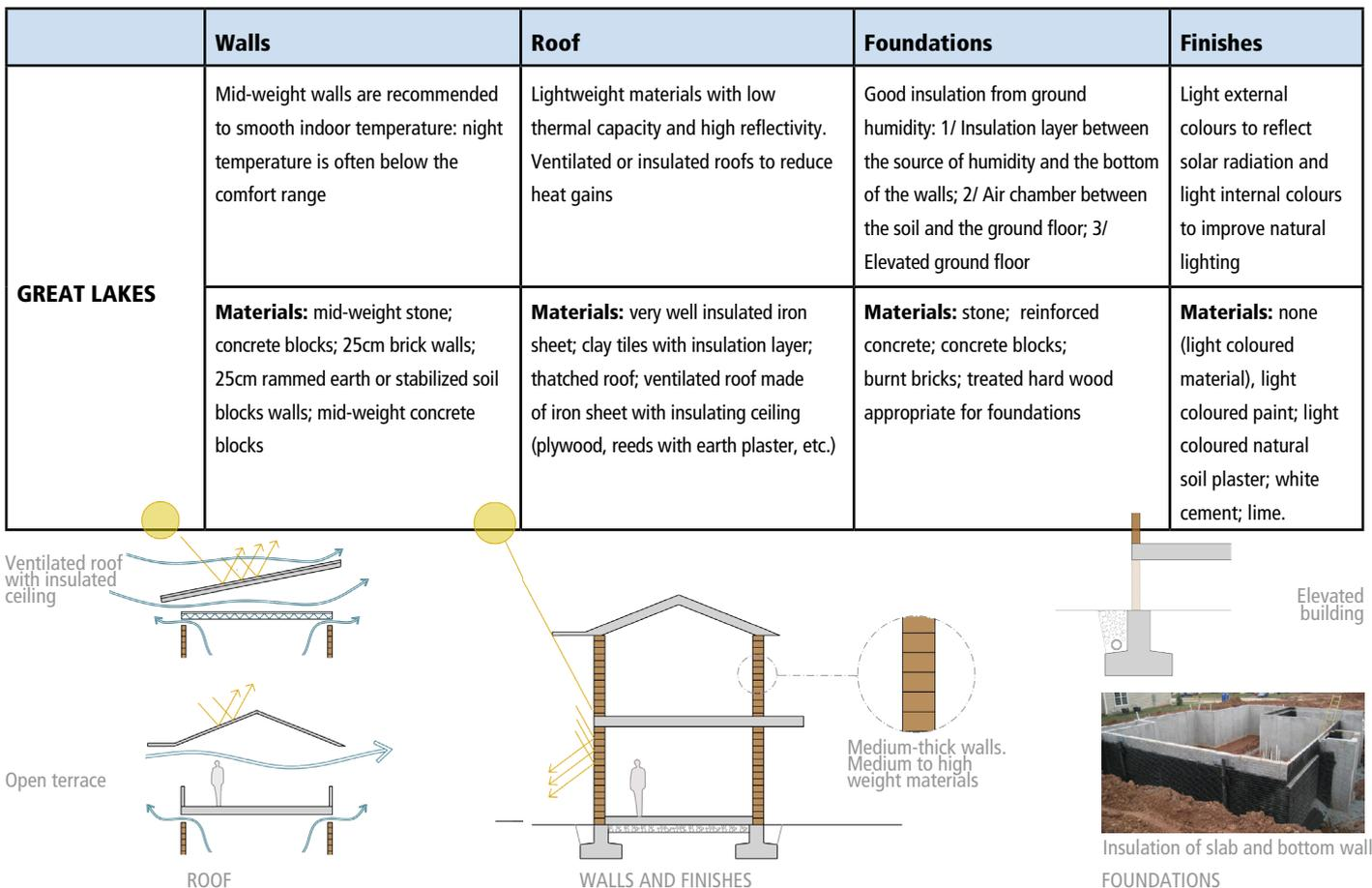
Fig. 10: Building materials appropriate for hot and arid climate
