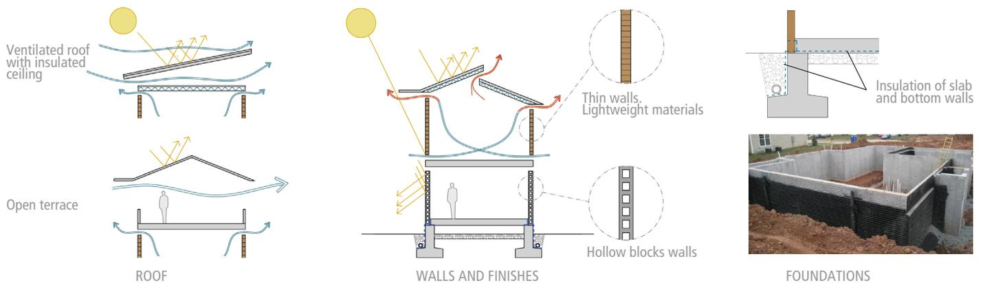
Fig. 07: Building materials appropriate for hot- semi arid / savannah climate
