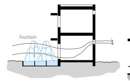
Fountains, sprays, pools and ponds are particularly effective passive cooling techniques. Hot air is channelled over the water before it enters the building.
