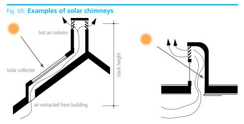
The heated air rises and escapes to the outside. This causes internal air to be pulled into the heated space and expelled thus enhancing airflow.
