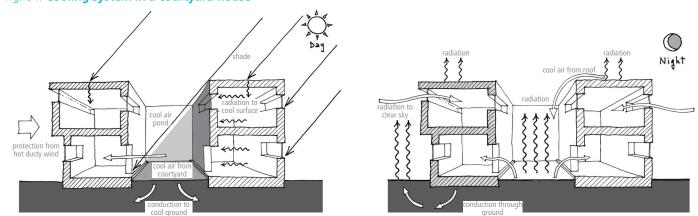
Courtyards are excellent thermal regulators. High walls cut off the sun, except for around midday, and large areas of the inner surfaces and floor are shaded during the day. During the night the heat accumulated during the day is dissipated by re-radiation.
