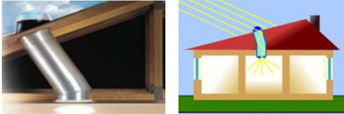
These systems bring daylight indoors. They are highly energy efficient due to the direct use of natural light, and the collection and diffusion of light without the consumption of kinetic energy as there are no moving parts such as sun tracking devices. Mirror ducts are low maintenance due to a simple, sealed structure that protects them from failure and deterioration.
