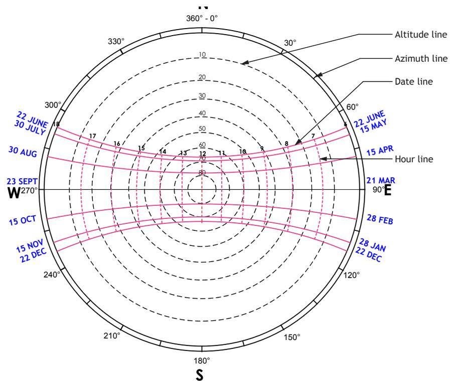
Solar control through shading devices is most effective when designed specifically for each façade, since time and duration of solar radiation vary with the sun's position in the sky - its altitude and azimuth.
