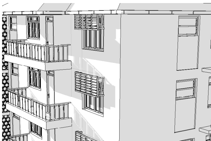
Figure 5: Horizontal louvres on vertical plane
