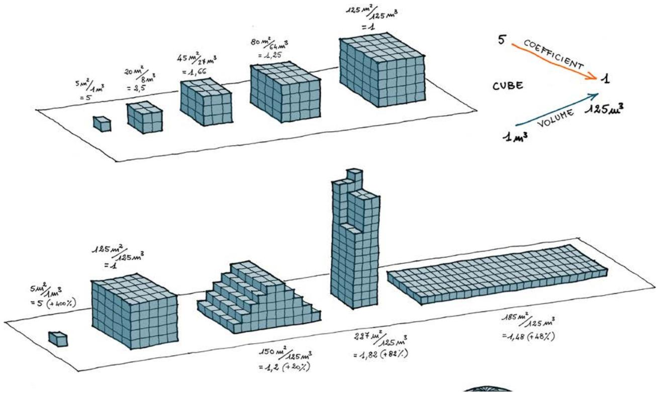
Fig. 2.18 Variation of surface to volume ratio (S/V) for increasing volume of a cube.
