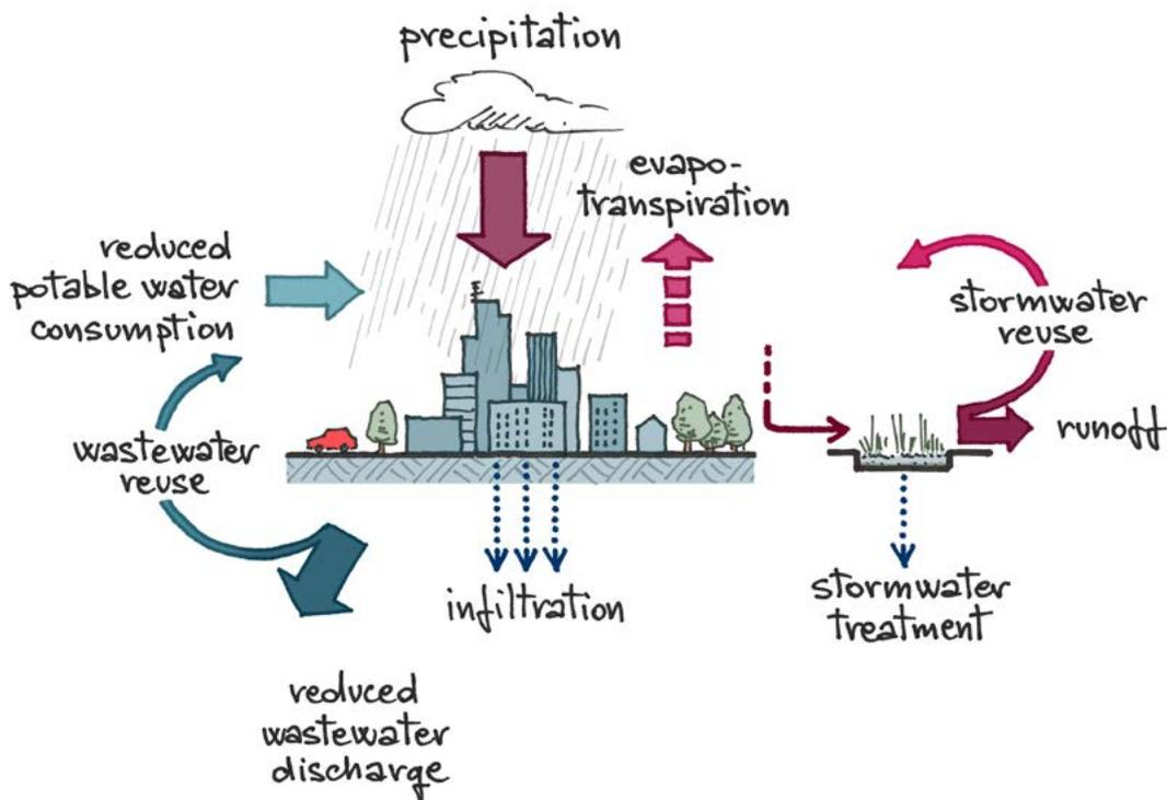
Fig. 2.25 The ideal water cycle of a settlement
