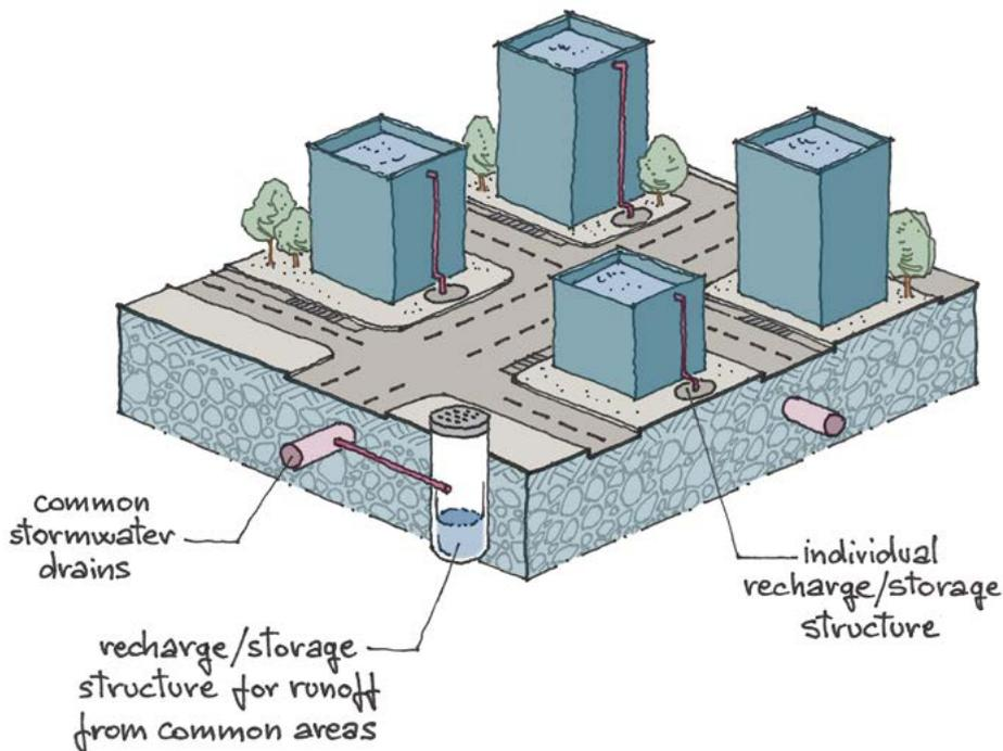
Fig. 2.26 Rooftop rainwater harvesting system
