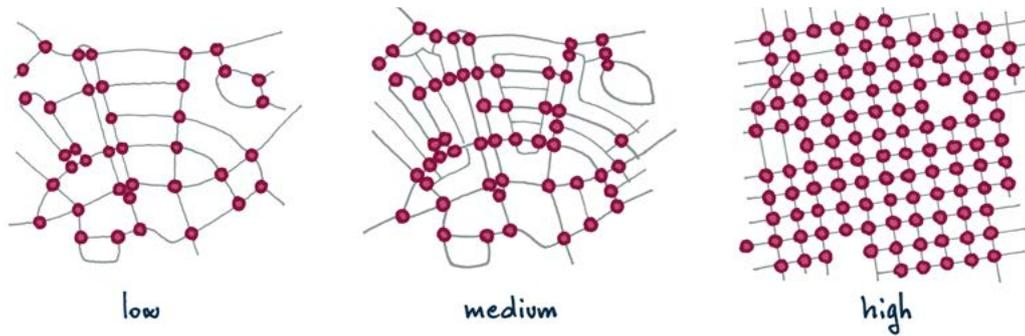
Fig. 2.5 From left to right: increasing connectivity index. A well-connected road or path network has many short links, numerous intersections, and minimal dead-ends. As connectivity increases, travel distances decrease and route options
