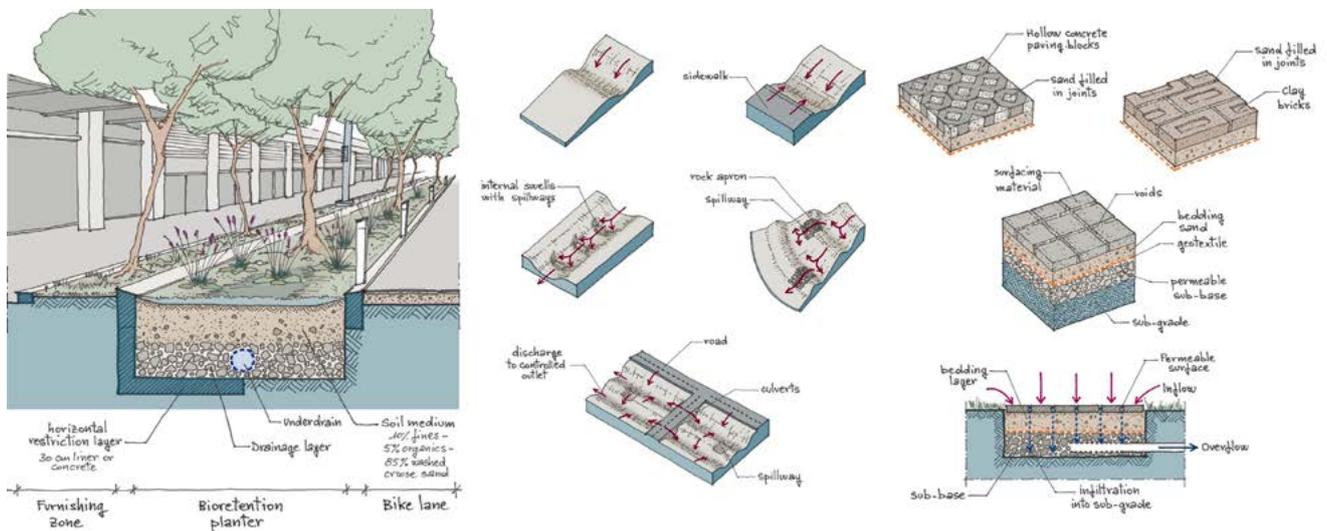
Fig. 2.29 Microbasins, swales and porous pavements
