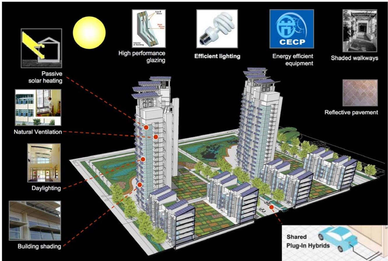
Fig. 2.49 EcoBlock’s technical system
