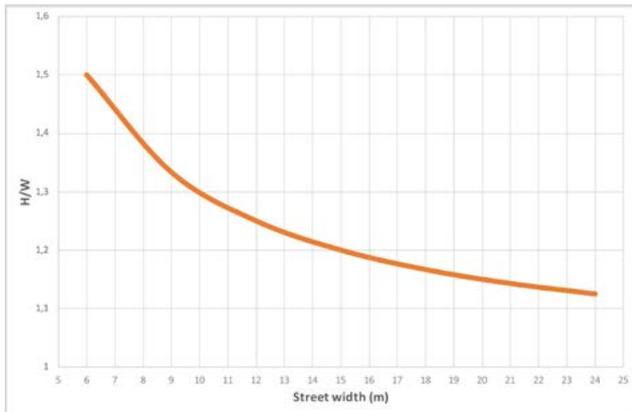
Fig. 2.14 Canyon H/W ratio to achieve full sun exposure on 21 December between 10:00 hrs and 14:00 hrs from 1st floor upwards as a function of street width, at the latitude of Yangtze river delta (30-31° N latitude)
