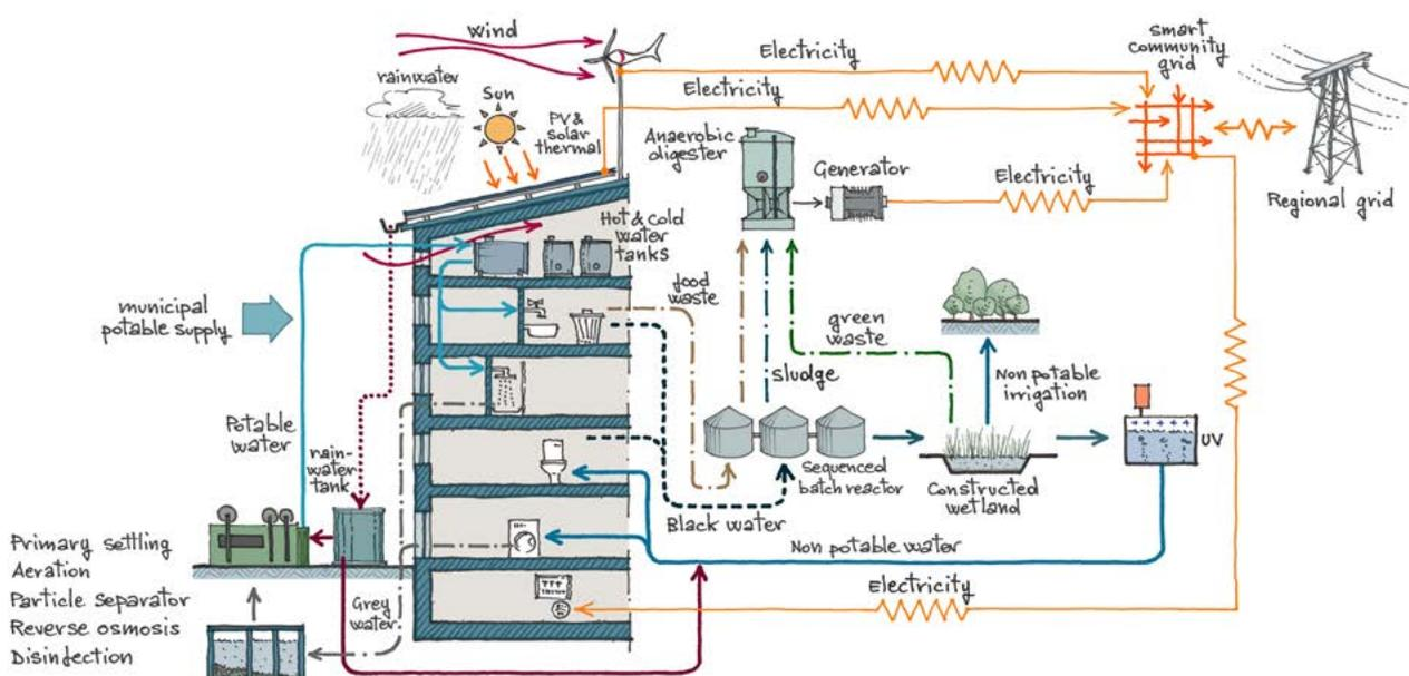
Fig. 2.37 Schematic of a building integrated into the zero carbon village's water, waste and energy systems
