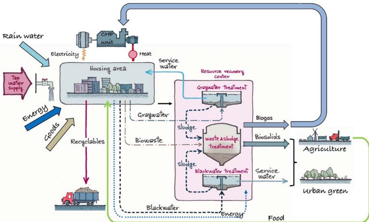
Fig. 2.36 The ideal waste and wastewater system, producing energy
