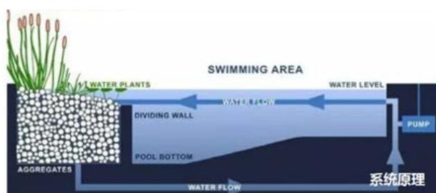
Fig. 3.29 water purification pool system
