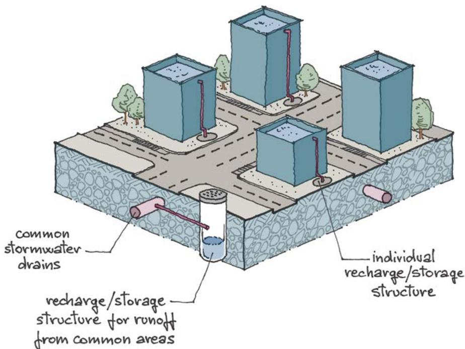
Fig. 2.26 Rooftop rainwater harvesting system
