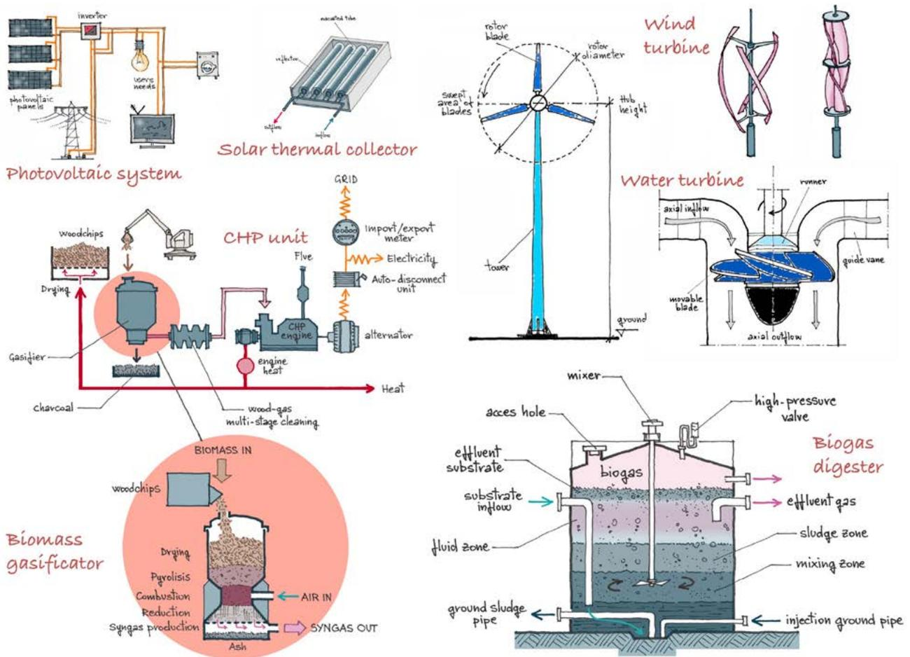
Fig. 2.22 Renewable energy technology suitable to supply a zero carbon village: Solar PV, solar thermal, mini and micro wind turbines, mini hydro plants, biomass gasification unit combined with an internal combustion engine driving an alternator for providing electricity and heat, biomass digesters for biogas production from sewage water and food waste, to be used also in a CHP system.
