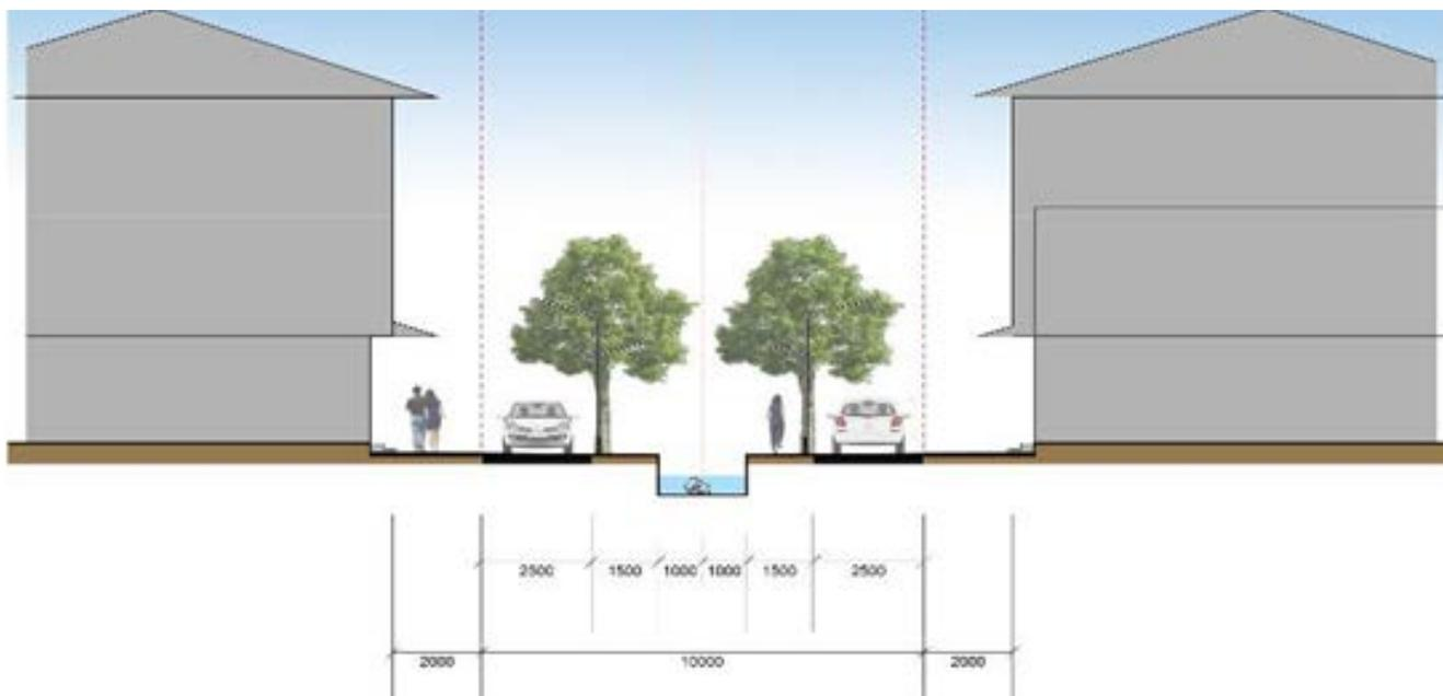
Fig. 3.7 Section of the newly planned roads in Shatan village
