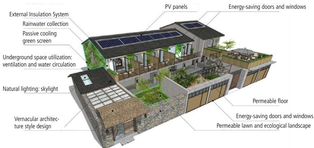
Fig. 3.10 Energy efficient technologies used in the adaptive reuse of 'Liangsu'
