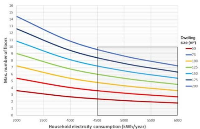
Fig. 2.23 Relationship between annual electricity consumption of an average dwelling in a building and the maximum number of floors in the same building for balancing the annual consumption of all dwellings, for different dwelling sizes. Calculation for Shanghai (Pudong Airport) solar radiation data.
