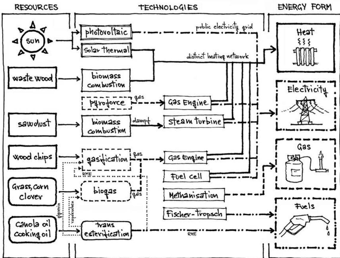
Fig. 2.53 Güssing energy system
