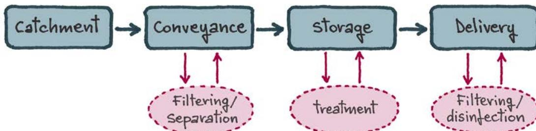
Fig. 2.27 Rainwater harvesting: process diagram for drinking water
