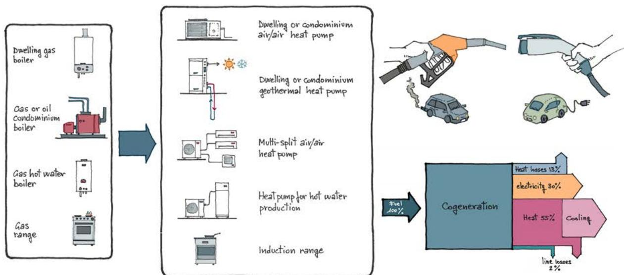
Fig. 2.21 Shift towards electricity driven energy conversion technologies and CHP.
