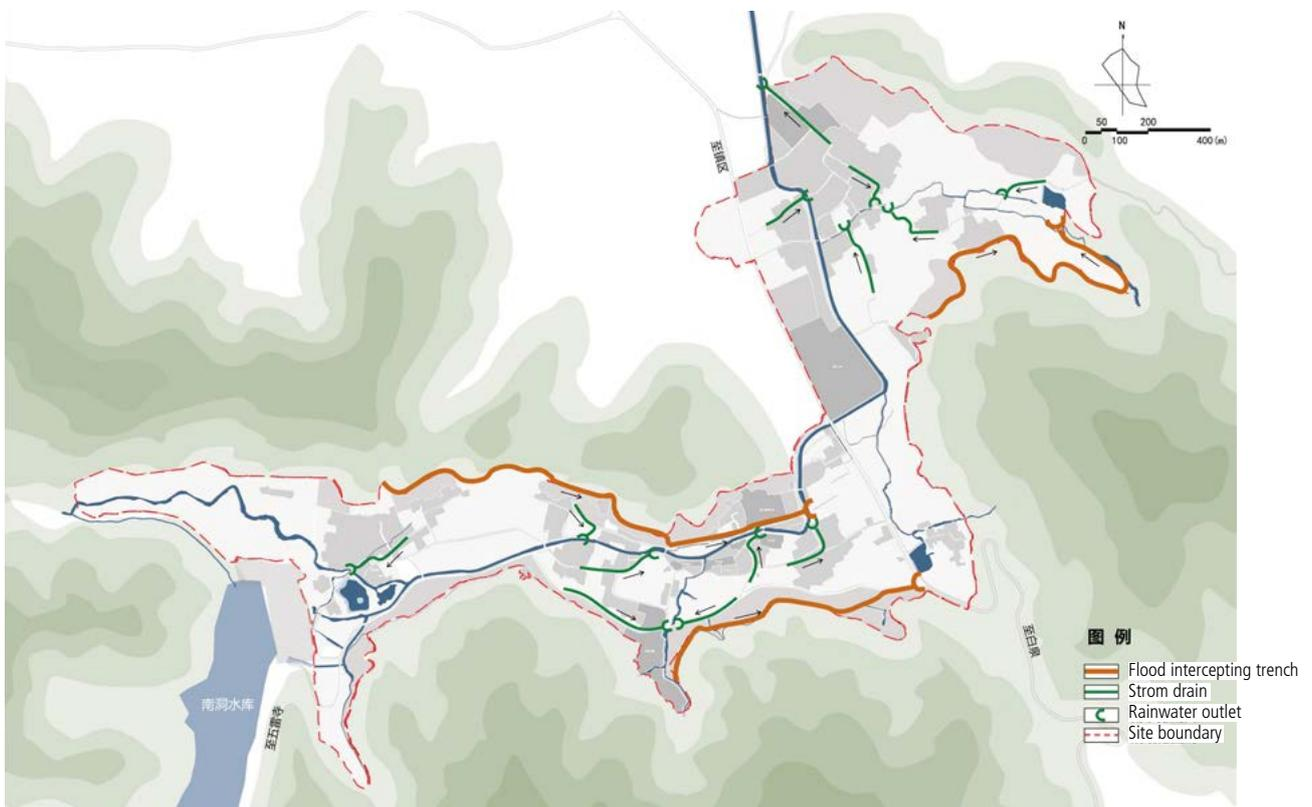
Fig. 3.28 Flood discharge channel, rain channel and flood cutting ditch
