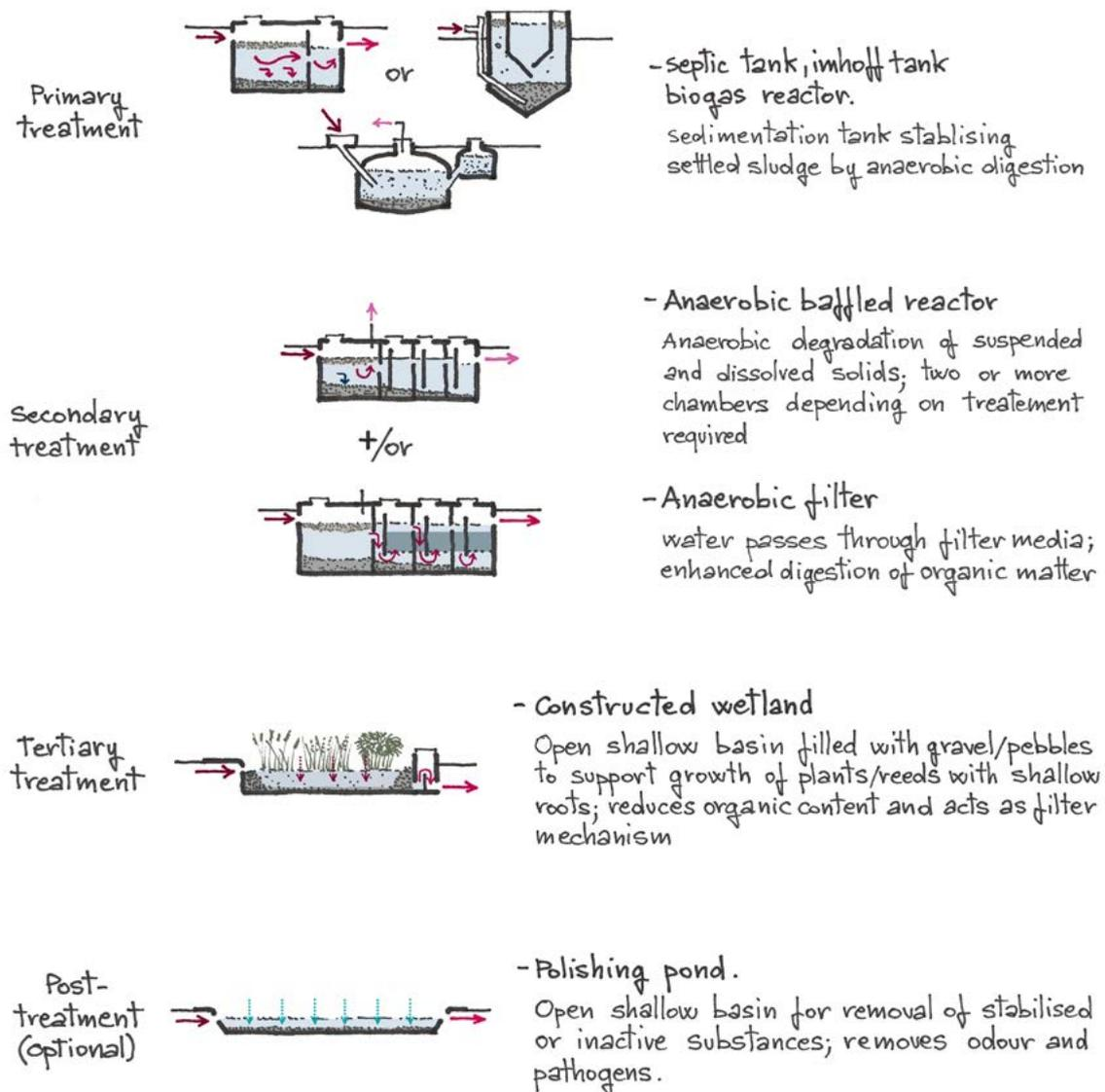
Fig. 2.32 DEWATS configuration scheme suitable for small-scale decentralized wastewater treatment<sup>67</sup>
