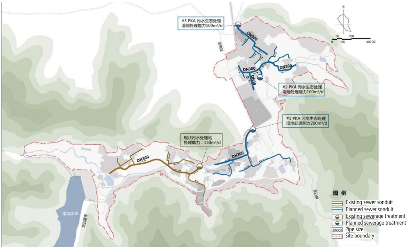
Fig. 3.27 Waste water system plan
