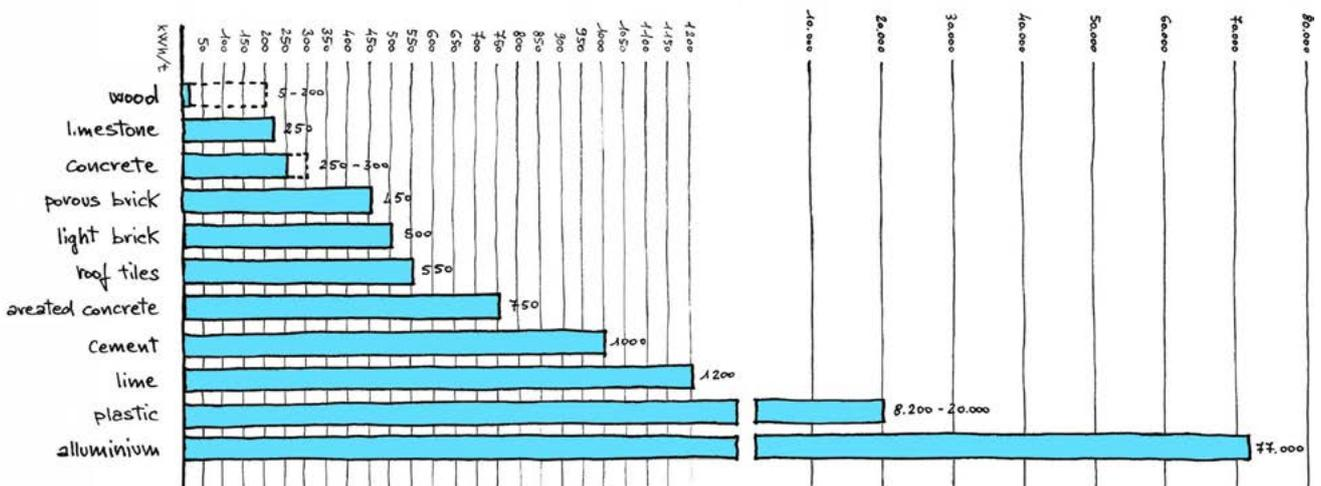
Fig. 2.17 Embodied energy for selected building materials<sup>59</sup>
