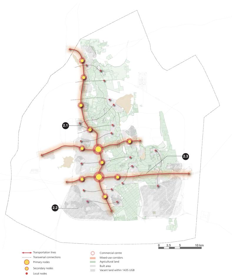
Fig. 45. Action 2: Implement strategic densification around main nodes and transport lines
