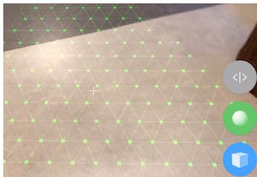
**Early block builder prototype:** Creating a 3D map of the physical environment, which is not normally visible to the user.
