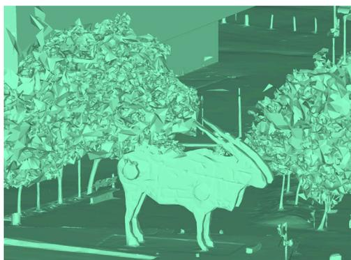
**3D model:** One example of a point cloud converted to a basic 3D mesh.
