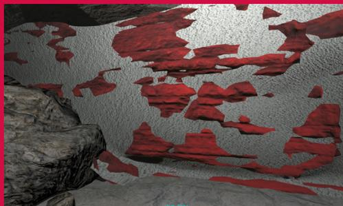
**Mixed reality mining:** Operators of mining equipment are guided in the reinforcement of tunnels. The red parts indicate that a thicker layer of concrete is needed.
