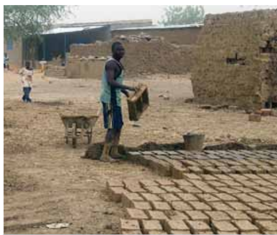
Sun-dried brick production for self-help housing processes in Chad © UN-HABITAT
