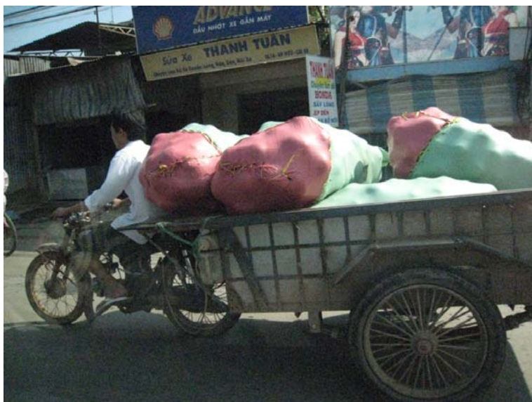
Figure 14. Motor-cycle converted to goods van in Ho Chi Minh City, Viet Nam
