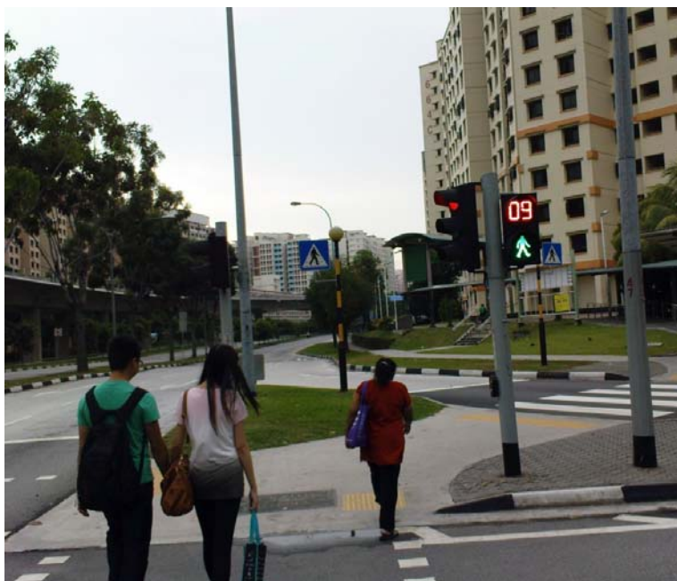
Figure 3. Pedestrian crossing system with electronic timer display in Singapore
