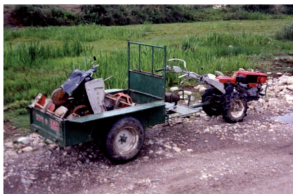
Figure 7.6 and Photo 7.6 Low-cost two-wheel tractor adapted for waste collection
