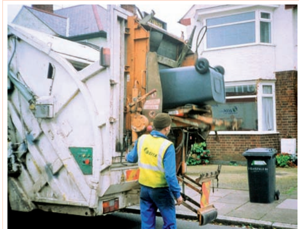
Photo 7.19 Compactor truck with binlift
