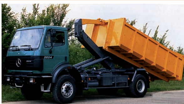
Photo 7.28 Hooklift truck loading open container
