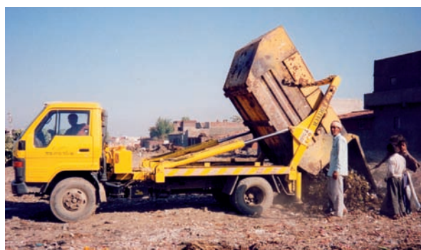
Photo 7.27 Skiplift truck discharging load
