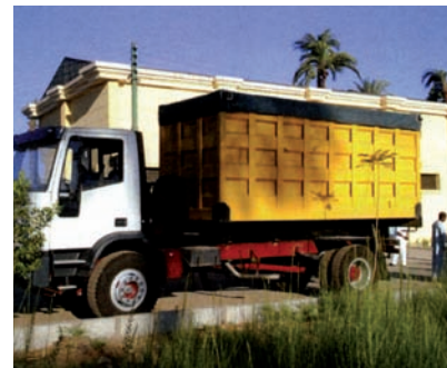
c) Container on specially designed tipping transport vehicle. Container capacity to suit waste density and truck load rating.
