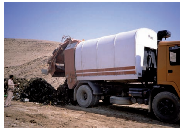
Photo 7.21 Rotating drum truck unloading
