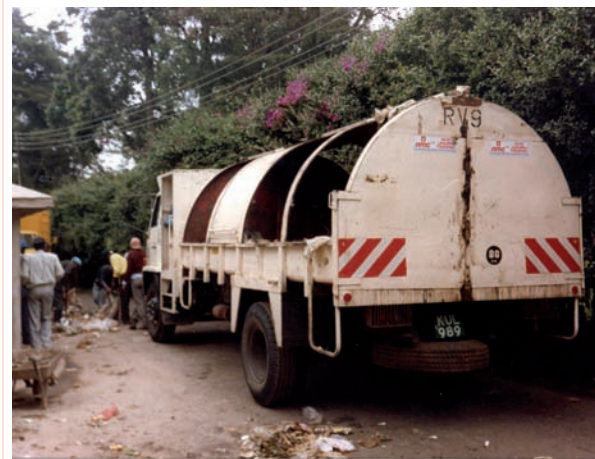
Figure 7.13 and Photo 7.12 Roll-top collection vehicle (side loader)
