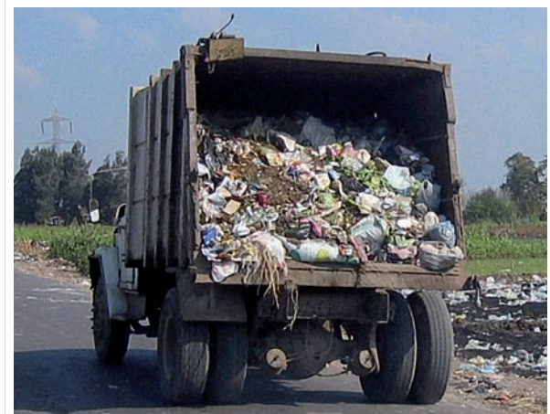
Photo 7.20 When the compaction mechanism cannot be repaired it can be taken off
