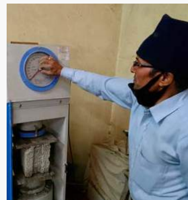
Block testing taking place at the Central Material Testing Laboratory in Nepal. Source: HRRP.
