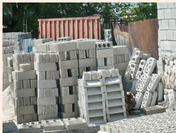
Low-quality blocks for reconstruction. Haiti. Source: UN-Habitat.
