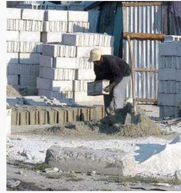
Low-strength blocks will affect compliance with standards. Source: UN-Habitat.
