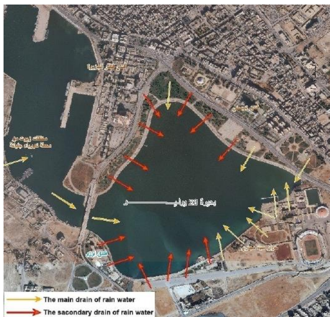
Rain water and sewage discharge to July 23 rd lake. Source: 3 rd generation master plan
