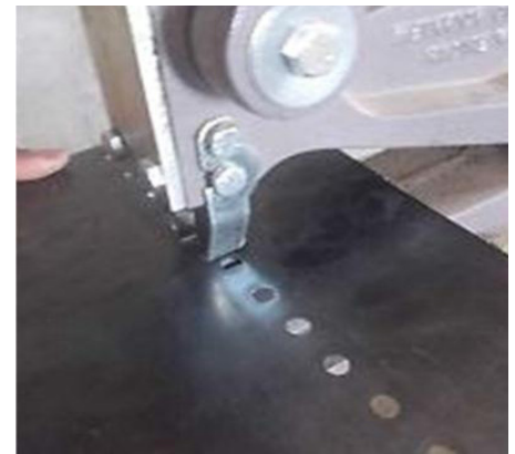
Step 3: Punch the holes in the sheet metal.
