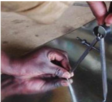
Step 1: Mark out the dimensions of the various stove pieces.
