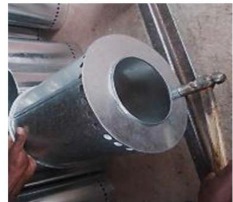
Step 6: Put a seam around the inner edge of the bottom cowling and then join it to the cylinder using the single bottom seam.
