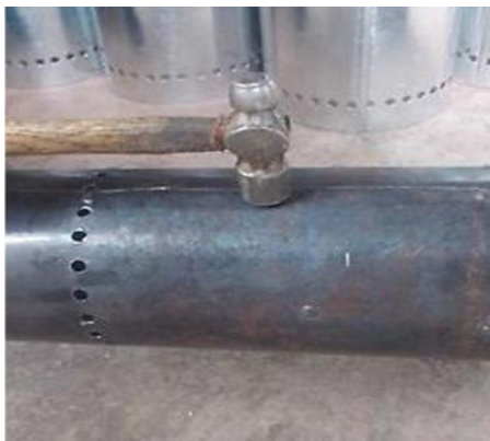
Step 5: The 2 ends of the fuel chamber are joined as well as the cowling. The lap seam requires riveting as well. Steel rivets should be used.
