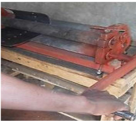
Step 4: Roll up the fuel chamber to form a round shape using a slip roll. The outer cowling will form a rounded cylinder without requiring any tool. Bring the two ends together.
