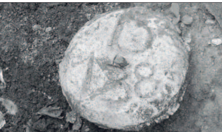
Figure 34. A cadastral survey peg - a steel rod, surrounded by concrete with the peg number incised
