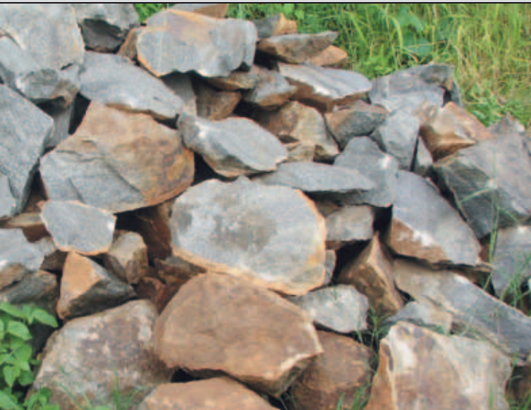
Figure 50. Hand split rubble
