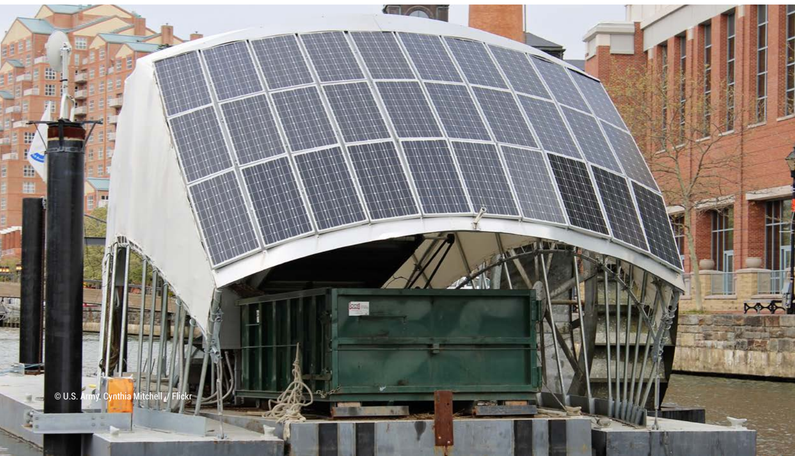
Figure 15: Baltimore, USA. The Inner Harbor Water Wheel combines old and new technology to harness the power of water and sunlight to collect litter and debris flowing down the Jones Falls River. The river’s current provides power to turn the water wheel, which lifts trash and debris from the water and deposits it into a dumpster barge. When there is not enough water current, a solar panel array provides additional power to keep the machine running. When the dumpster is full, it is towed away by boat, and a new dumpster is put in place.
