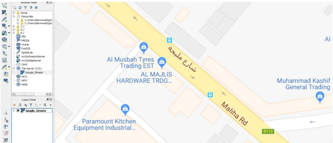
Figure 3: Google streets tile server in QGIS can be used to identify location of public transport stops
